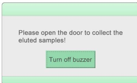
Once an elution step is complete, the instrument will buzz and a popup message will be displayed. After the elution is completed, open the safety door and the platform will come out automatically. Collect the eluted samples using a pipette.
