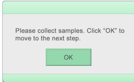
Once the user opens the safety door, the rack platform and magnets will come out automatically and a second message will appear at the same time. The user can remove the sample rack to collect the elution. If the user does multiple elution cycles, they may press OK after transferring the samples. The instrument will continue with the next elution step.
