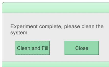
When the instrument finishes the method, the completion message window will appear on the screen to remind the user to clean the instrument and fill the pipelines before starting the next run or shutting off the instrument. The user can skip the step by pressing "Close" if there is another run.
