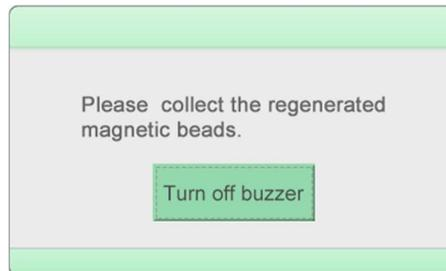
The message appears when the regeneration process is complete. The buzzer can be turned off manually.
