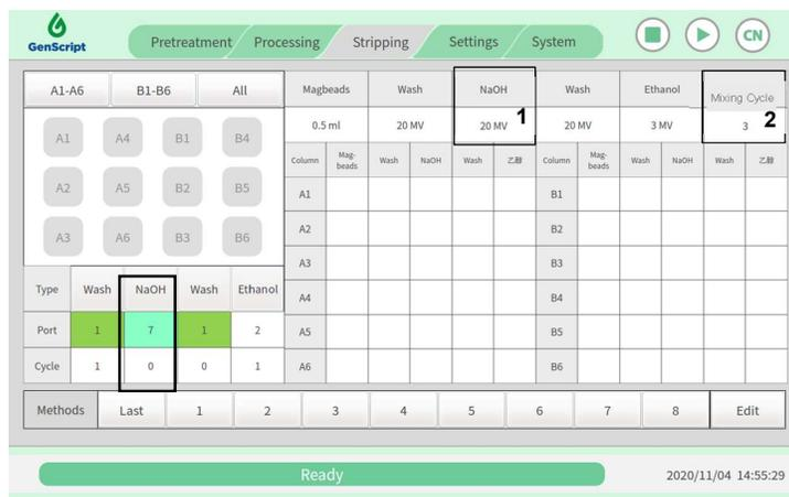
The regeneration interface has similar functions to the processing interface except that there are NaOH between wash 1 and wash 2 and NaOH Cycle instead of elution time. The two new processes in the stripping interface are highlighted in black in the above picture(1 and 2). NaOH solution should always be connected to port 7.
