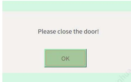
If the safety door is opened during an active instrument process, the message will appear and the instrument will automatically stop all its actions. The user needs to close the safety door to continue the interrupted process.
